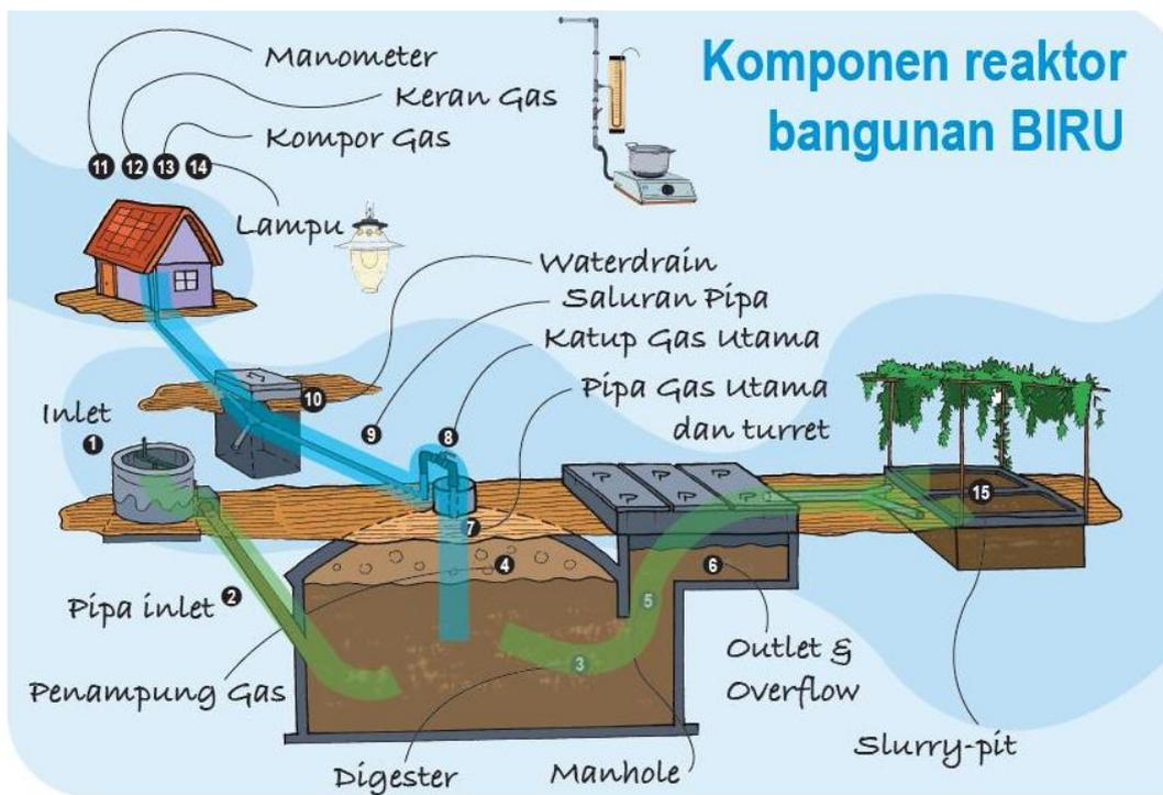
Figure 1. Reactor components of BIRU installation. 1. Inlet (mixing tank); 2. Inlet pipe (optional to be connected to toilet); 3. Anaerobic digester; 4. Gas storage; 5. Manhole; 6. Outlet and overflow; 7. Main gas pipe and turret; 8. Main gas valve; 9. Pipeline; 10. Water drain; 11. Pressure Gauge; 12. Gas tap; 13. Gas stove with a rubber hose pipe; 14. Lamp (optional); 15. Bio-slurry pit.
